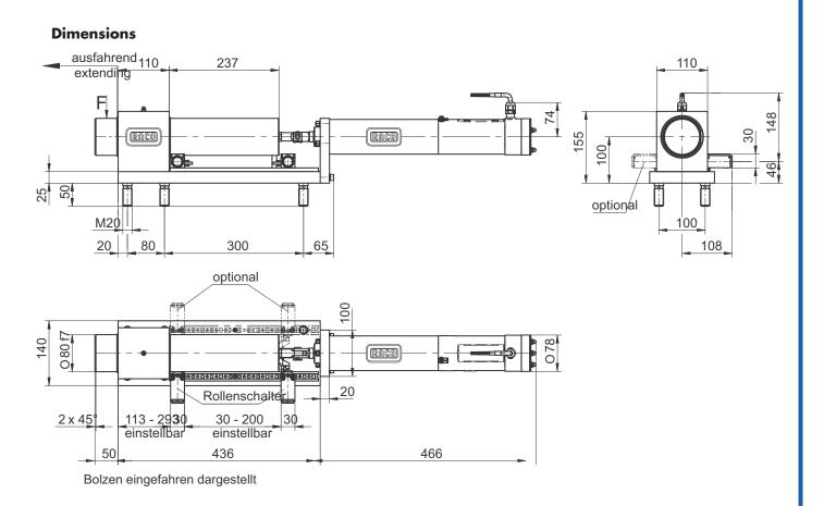
Max. load 5.000 kg per pin (recomendation: 4 Pins per cabine)
