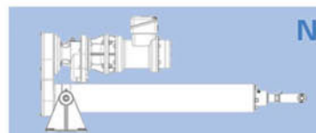
Type N Design: Electric Actuator with a RACO parallel Gear Motor and C Drive Housing
