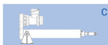
Type C Design: Electric Actuator with a RACO Motor and C Drive Housing
