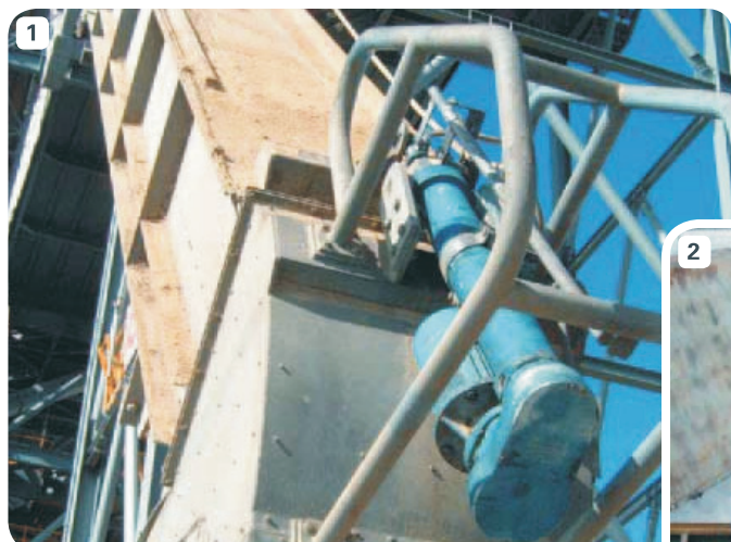
[3] Type T1A6 for a clam shell gate
