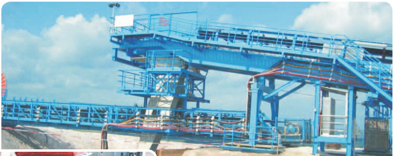
Chute in a conveyor belt feeder
