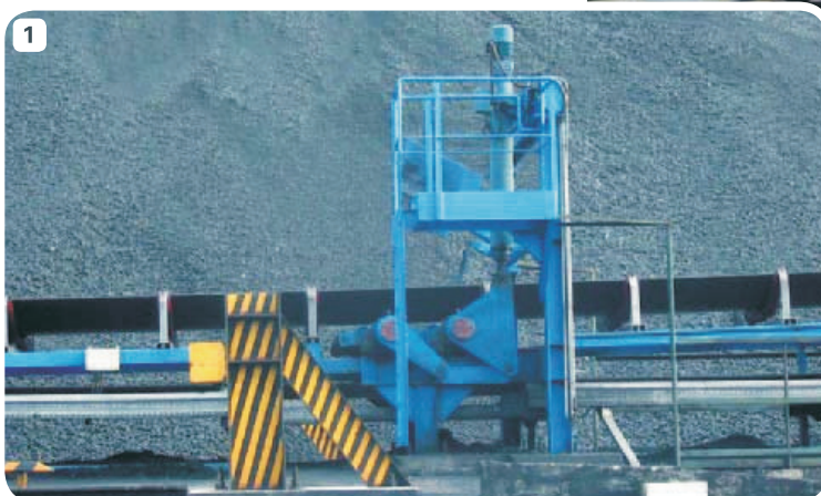
[1] Type T1M7 for a conveyor belt wiper (plough) [3] Type T1N7 for a gravity chute in brown coal open pit mining plant [2] Type T1M8 for a conveyor belt wiper (plough)
