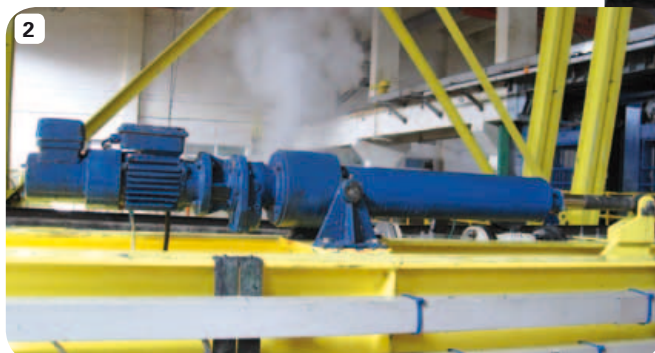
[1]-[3] Type: T1M5 / T1M6 Actuation of the grabber locking in an electroplating system
