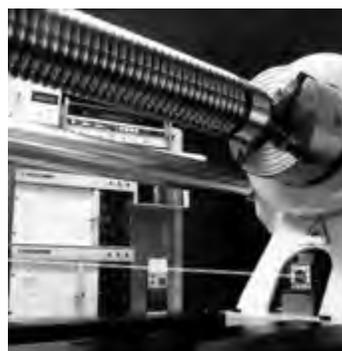
Fig. 25: Laser linear measurement equipment
